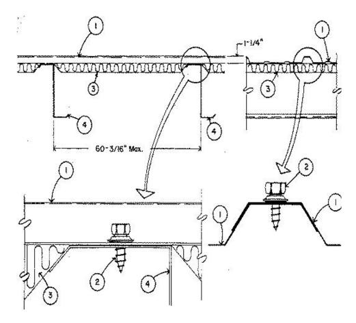
1. **Metal Roof Deck Panels\*** — No. 26 MSG min gauge coated steel. Panels continuous over two or more spans. End laps to occur over purlins with panels overlapped 3 in. min., 6 in. max with lap centered over purlin web. A line of tape sealant may be used at panel side and end laps.
